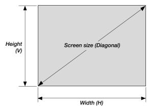
Formulas: Screen width H (m) = Screen Diagonal x 4/5 x 0.0254 Screen height V (m) = Screen Diagonal x 3/5 x 0.0254 Screen width H (inch) = Screen size x 4/5 Screen height V (inch) = Screen size x 3/5
